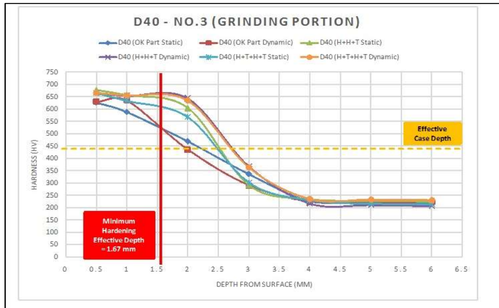
Gambar 4.1 Grafik Hardness area radius grinding (item no.3)
