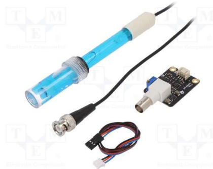
Gambar 1. Sensor pH (SEN0161-V2)
