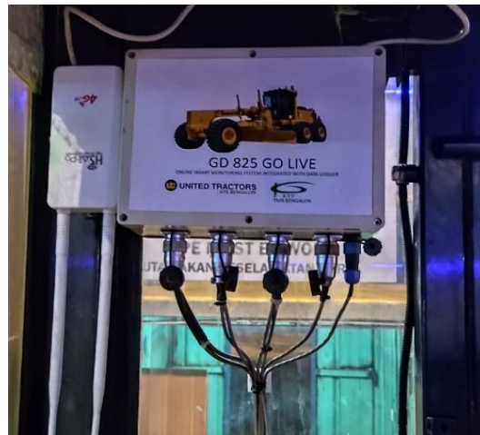
Figure 16. lot module ( GD825 GOLive ) installed to machine
