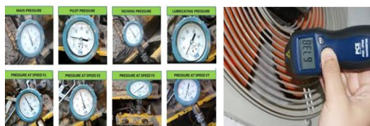
Figure 2. Manual measurement to determine engine & transmission health
