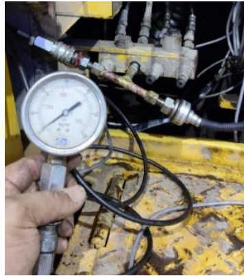
Figure 12. Calibration process for oil pressure sensor
